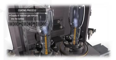
Plasma reaction with pulsed microwave and SIOX separation in vial.
